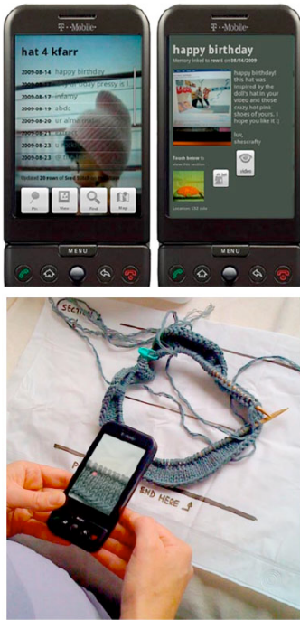
Figure 2. The current system (above) was developed for the Android 1.5 G1 phones and uses computer vision to correlate recorded media with locations on fabric. Marie's project for Kristin is shown on the Spyn screen.
